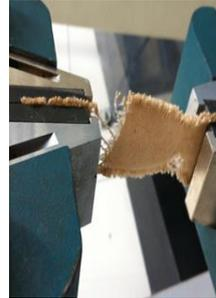
The strips are dried and sent to Roehampton where a machine (tensiometer) measures tensile strength decomposition. More decomposition means higher function in the hyporheic zone.
